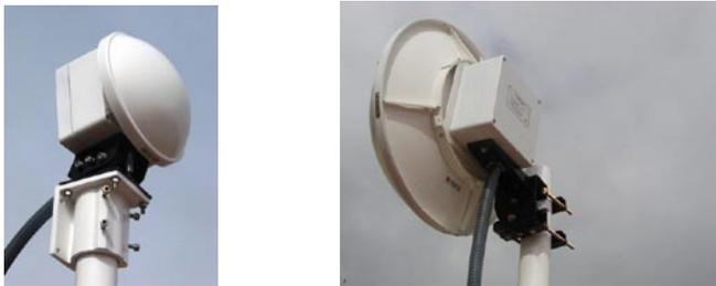
*Figure 6: AireBeam™ radio with smaller short distance (left) and a larger longer distance antenna.*
