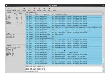
The user interface has five parts. The large window shows the decoded LI messages as they are received. The small window on the top left shows real-time statistics. The small window at the mid left shows state information. The small window at the lower left shows some of the current configuration parameters. Finally, the status window at the bottom shows status and error messages.
