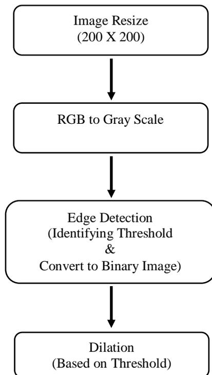
Fig. 2 Process Flow of Image Pre-processing
