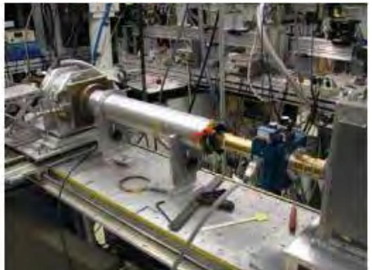
This is a small-angle setup on a laboratory source with an approximately 1 meter path length, the wavelength was about 1.5 Å. Based on this typical configuration one would expect at least down to  $q = 0.01$  ( $2\pi \sin(\theta)/\lambda$ ) or equivalently (d-spacing of maybe 600 Å).
