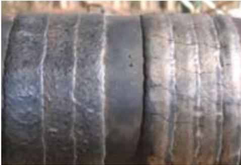
There are more differences than just esthetic appearance between a non-cracking and a cracking casing friendly hardbanding wire. Certain hardbanding wires crack because of the fine carbides that form on grain
