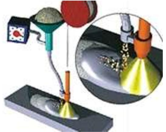
The mild steel welding wire acted as a matrix to hold the tungsten carbide particles. It was an easy choice since it was readily available. The tungsten carbide was used tool bits that were crushed to various sizes. However, as good as tungsten carbide is for abrasion resistance, the weak link is the soft mild steel matrix. As the mild steel matrix wears away during the drilling process, the tungsten carbide granules fall out.
