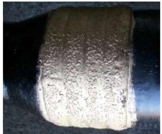
Duraband NC wire with Tungsten carbide particles
