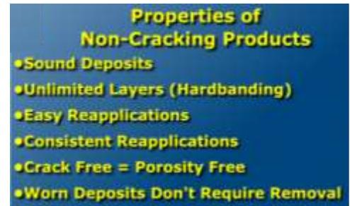
Product that does not crack, normally will rebuild very easy. In addition, as there are no cracks, foreign matter such as drilling fluids, abrasives and H<sub>2</sub>S cannot become entrapped, making reapplication even easier for the hardbander.
