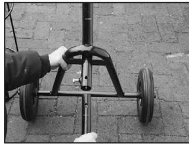
Step 3 Insert Draw Bar into Main Frame.
