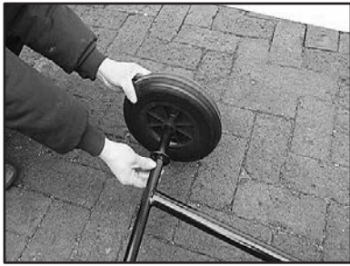
Step 1 Install Wheels on Lower Frame Unit
