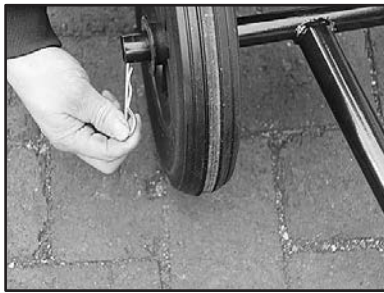
Step 2 Put on Washer and Snap on R-clip.
