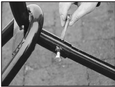
Step 5 Put in Bolt to Hold Main Frame to Draw Bar.
