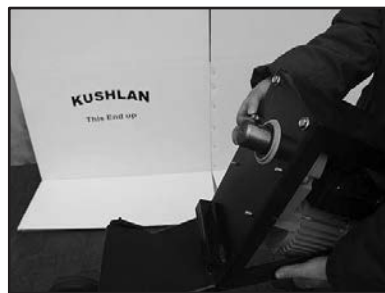
Step 9 Install Gear Motor with the Nuts and Washers. They were removed before
