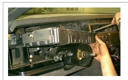
Disconnecting the dash harness to Cluster connectors is accomplished by lifting the metal security clips with a small screwdriver and wedging the connectors off with a flat blade screwdriver. The Cluster is free.
