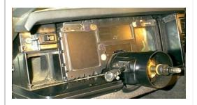
The photo to the left shows the Cluster exposed with the dash pad not lifted as yet. Remove or loosen four (4) 7mm screws holding the Cluster. Two alongside the Steering column and two at the upper corners of the Cluster. Tilt the steering column down and unscrew the tilt lever (counterclockwise).
