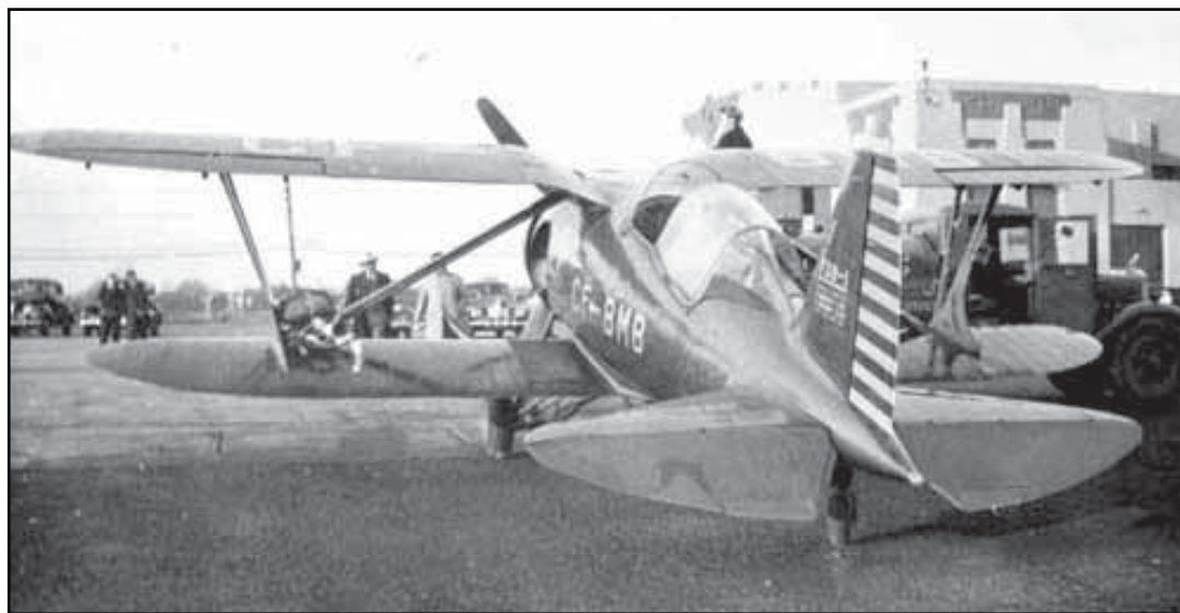
This 3/4 rear shot provides a good view of how the gull wing meets the fuselage. You can see why visibility was a big concern.
