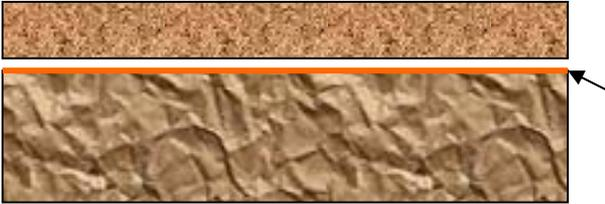
Aggrepave Polymer surface soaked 40mm depth 6mm to dust aggregate layer
