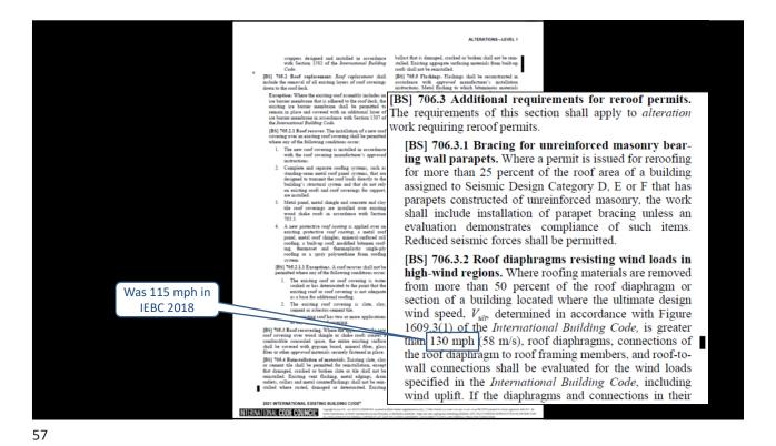
current condition are not capable of resisting 75 percent of those wind loads, they shall be replaced or strengthened in accordance with the loads specified in the International Building Code.
