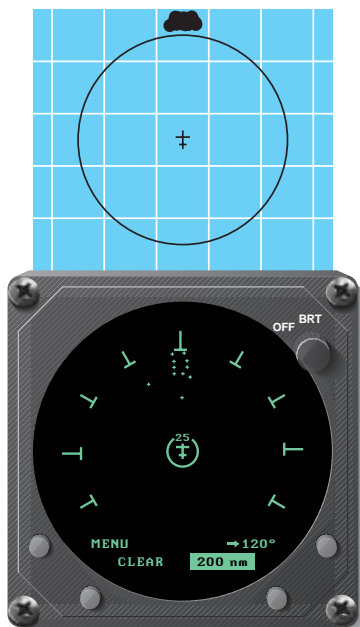
Figure 4-11. Discharge Points Off the Aircraft's Nose
