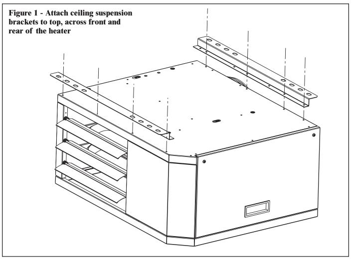
The heater may now be lifted and attached directly to the ceiling structure using a minimum of two anchor points per suspension angle.
