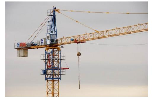
This is usually he first thing you will notice in the air as you drive by new construction sites. It is typically constructed to the highest floor of the anticipated building. It is needed to lift very heavy items quickly to the top of the upper floors of a building. Notice the counter weights at the top that are designed to balance the maximum load being hauled.
