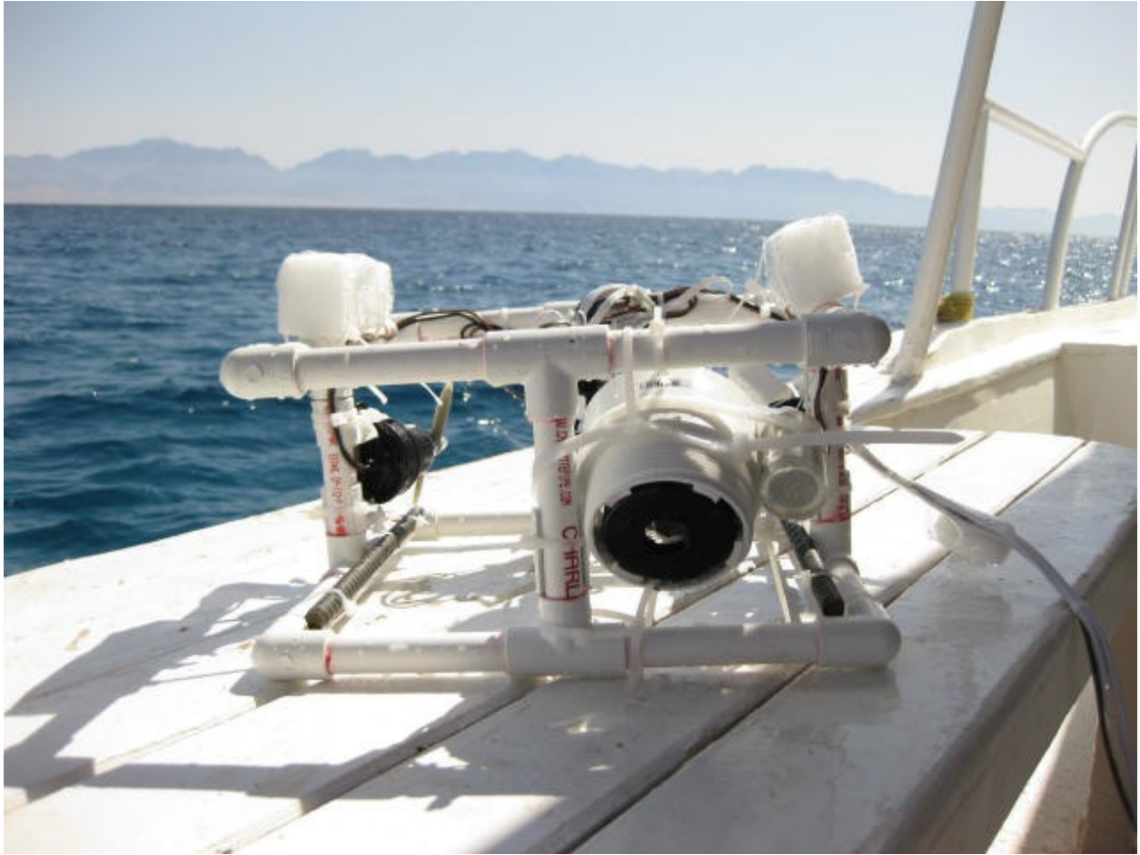
Above: I was able to make this ROV from a kit which had three motors and a video camera.
