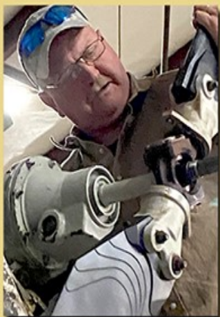
Exhibits Specialist Zane Mohler attaching the tail rotor on the Cobra
