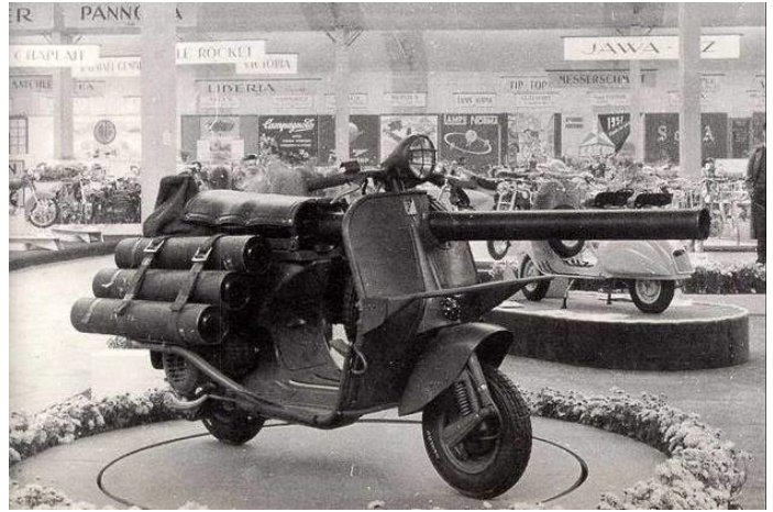
The Vespa 150 TAP is an anti-tank scooter with an M20 75 mm recoilless rifle made for French paratroopers.
