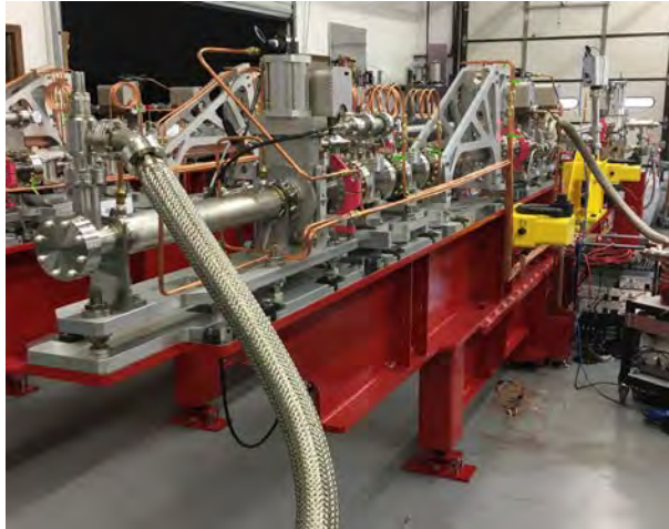
FIGURE 6: Front end undergoing leak testing; viewed from the upstream end.
