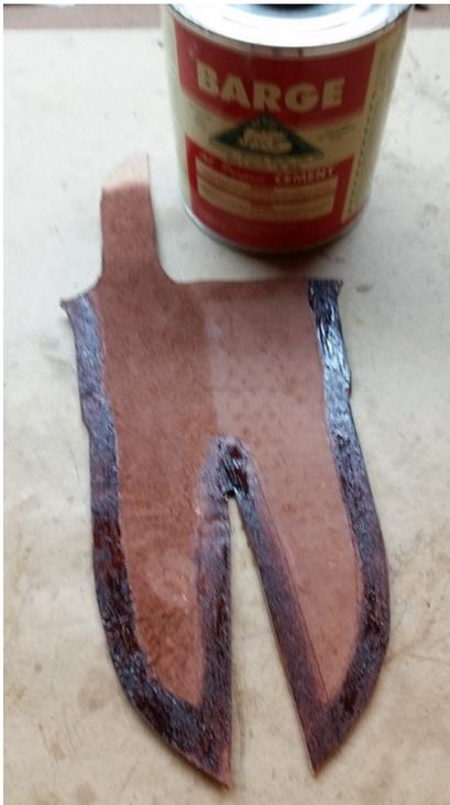
All of our parts are cut out and ready for tooling or glue up. I did tool the front of this sheath but that is not part of this build so I will skip that and maybe to it in a future article.
