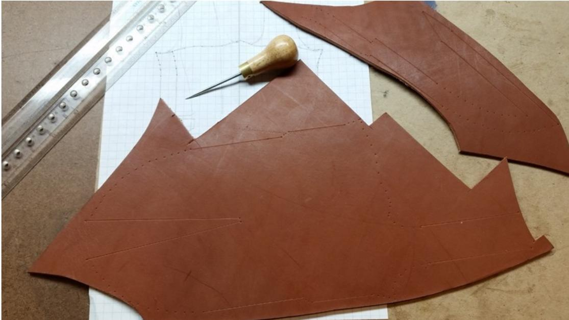
All of the pieces have been punched thru our pattern and onto the leather. Now it's time to cut out all of the parts to make up our sheath. I found that using a hole punch at the top of the foot will give you a nice clean fold.
