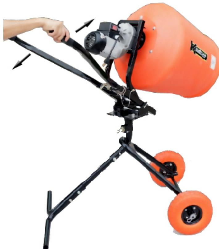
**INSTRUCTION** - Rotate the swivel latch 180° to the lock out position. To dump, raise the handles and dump the concrete out onto either a wheelbar- row or directly onto the work you are doing. By pulling the swivel latch and rotating at 180° to the lock out position, the mixer will rotate 360°.
