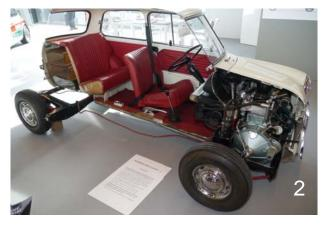
Photo 2- Cross section Mini from BMHT Gaydon.
