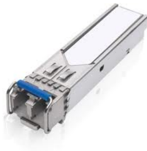
Figure 5.19 A typical SFP module
