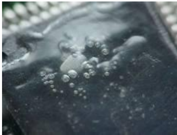
Figure . Voids and bubbles in conformal coating
