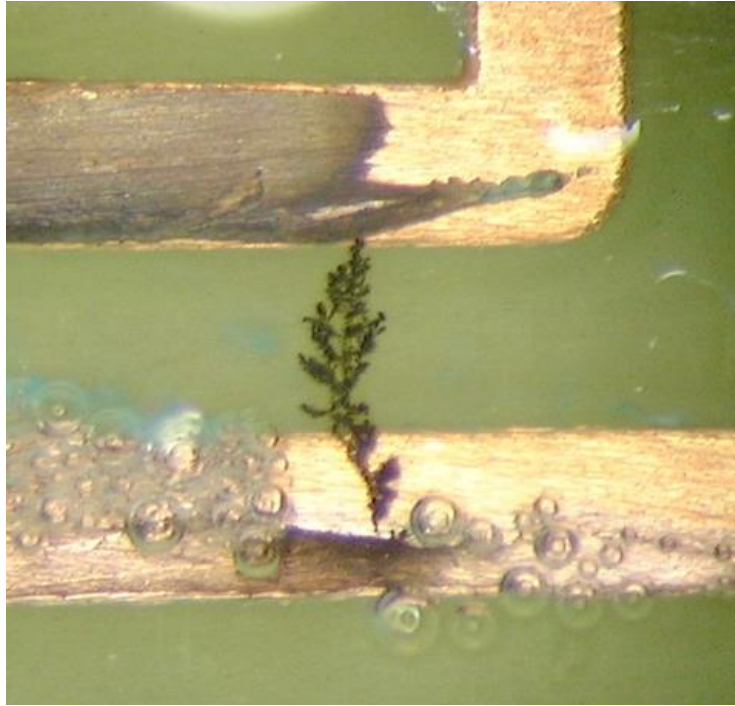
Figure . Dendrite bridging two PCB traces
