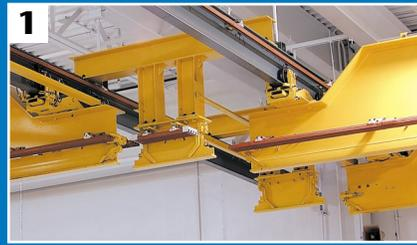
1. Both bridge girders approach the crossover track. The operator pushes a button powering a gear motor that activates a pair of rollers.
