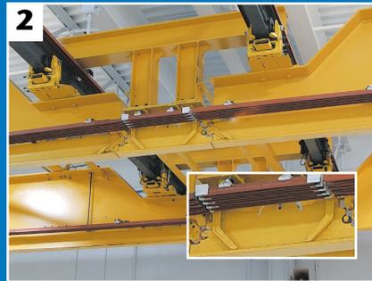
2. The bridges line up with the crossover track. The rollers move from the interlocking beam toward a wedge type engaging mechanism on the crossover track (see Photo 2).
