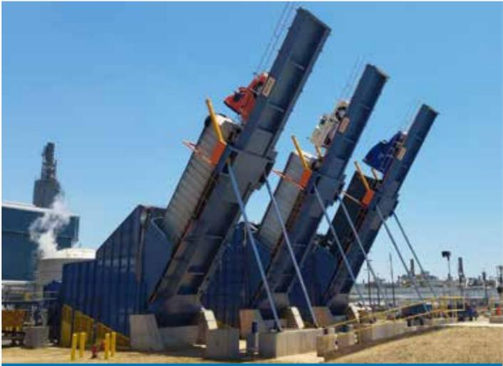
Truck rail and barge unloading system
