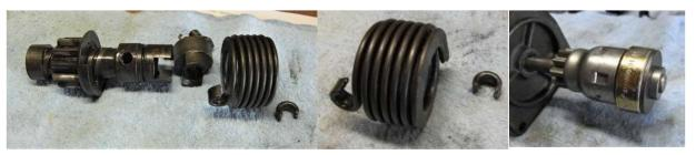
I read somewhere these modern drives are very reliable, we'll see! I would suggest carrying a spare starter drive spring about \$8, or the whole assembly for \$25, or the modern one for \$40 in your tool box of parts for peace of mind while driving around! Remember, these parts are over 90 years old!!!
