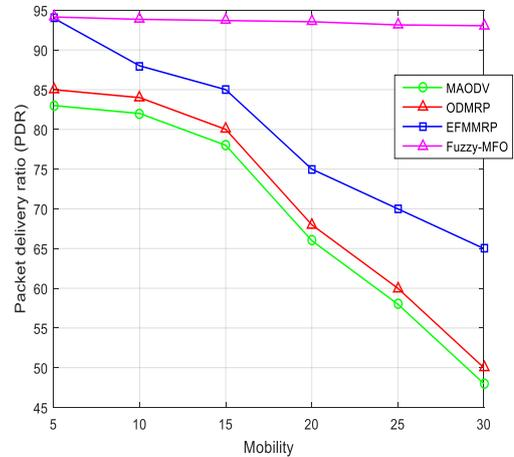
Figure 5 Comparison of Packet Delivery Ratio on the basis mobile nodes in network.
