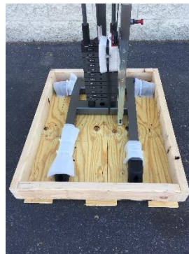
Pulley is zip-tied to the skid
