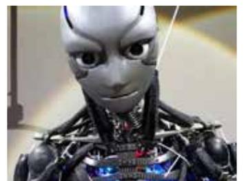
When the machine is powered, the actuators or motors pull these wires and trigger human-like muscle expansion and contraction, leading to the action associated with it.
