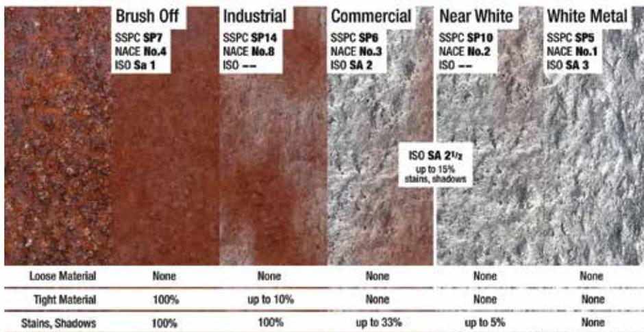
Figure 5. NACE/SSPC surface finishes, grades of blast cleaning (Adapted from ISO 850-1).
