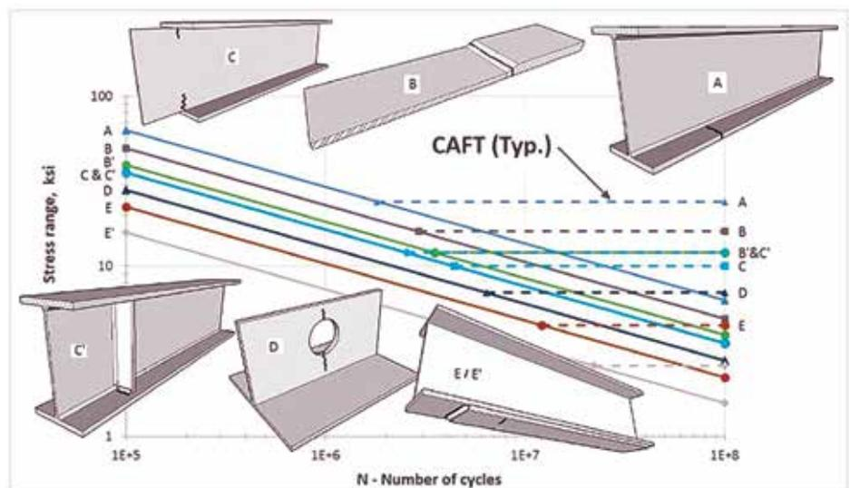
Figure 4. AASHTO Fatigue Curves (U.S. DOT, *Design and Evaluation of Steel Bridges for Fatigue and Fracture*).
