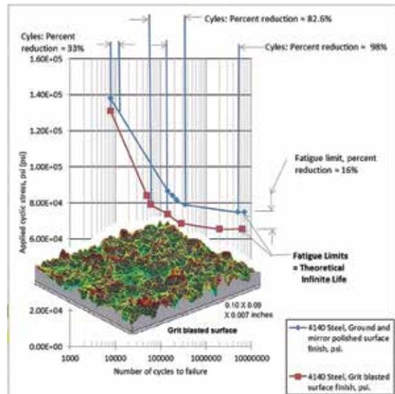
Figure 1. Grit blasting effects on 4140 steel before thermal sprays (Adapted from K. Padilla, et al.).
