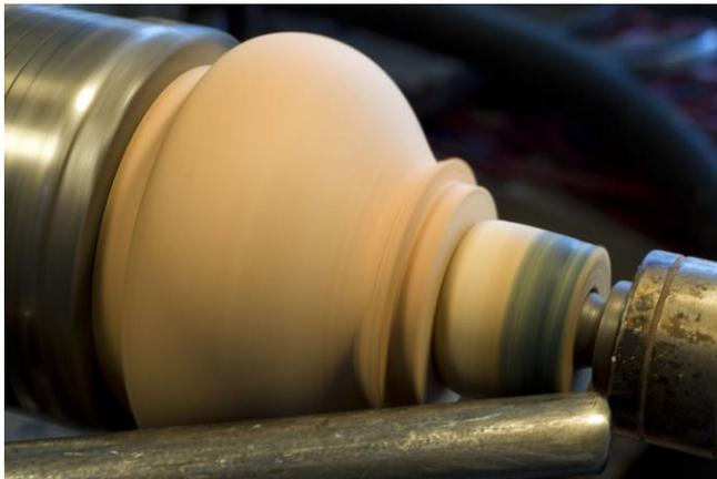
between the chuck jaws and the finished interior of the lid to ensure that the inside surface does not get damaged by the expanding chuck jaws. To ensure that the lid does not fly off the chuck, it is a good idea to bring the tailstock up to add a small measure of safety. Since I want to make the dome’s point as high as possible, I do not want to push the point of the live center into the center point of the lid, so I made a cover to fit over the point that has a
