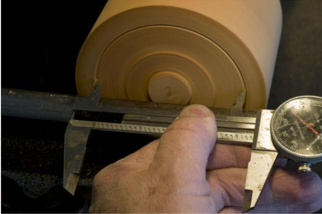
concentric circle. This is your line of absolute inside diameter and should not be crossed if you want the lid to properly fit the base. To ensure that you do not cross this line, use your 1/16<sup>th</sup> inch parting tool and cut a kerf into the base that is about 1/16 inside of the line that you just scored with the calipers. This will allow you to sneak-up on the final diameter of the hole and give you more of a probability of
