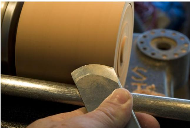
To ensure that I make clean cuts, I like to use my curved edge skew, which I hold flat on the tool rest. This tool, when used properly, can provide a surface that is clean and smooth, reducing the amount of sanding that is required. To make the base wider than the top, watch the top edge of the work piece as it spins. You will be able to see how your skew is shaping the edge as you move from the bottom toward the
