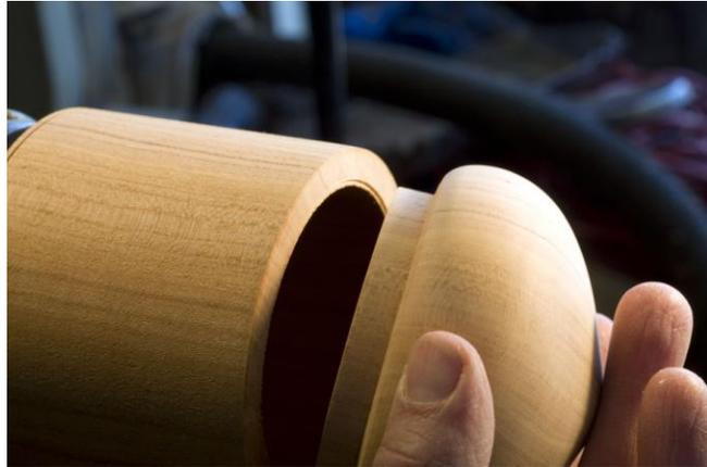
base all of the way around the rim. At first the fit will be tight – that is OK, because you still need to lightly sand the inside of the base.
