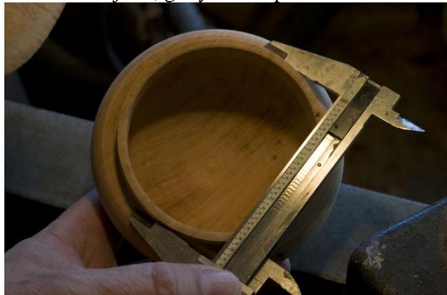
Next, you need to transfer the measurement to the top of the base. Move the tool rest up to the flat surface of the base and set it so it is about 1/16<sup>th</sup> of an inch below the centerline. Turn on the lathe at a medium speed and lay the calipers on the tool rest without engaging the wood. Your calipers should have two metal points that are exactly
