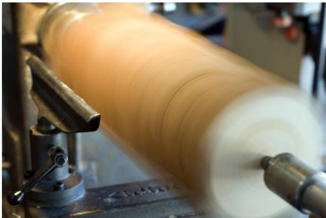
Find the center of each end of the piece of wood, make a mark or a divot to make it easy to find while holding the piece up to the lathe's drive center for mounting. Mount the piece of wood by pinching it between the drive center on the headstock and the revolving center on the tail stock. It is important that you spin the work piece a few times before you turn the lathe on to make sure the piece moves freely and does
