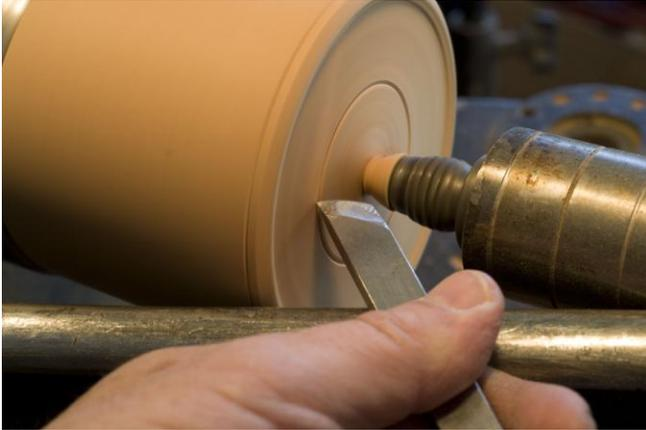
does not have to be used as I am trying to get as deep into the center of the base possible to reduce the remaining nub to a very tiny point by the end of the process.
