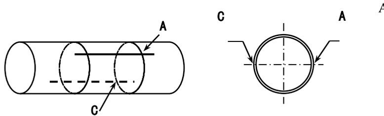
Remove the positioning paper, start from point C, and measure the installation distance L on the drawn straight line to determine point B. In this way, points A and B are the installation positions; for example, L=280mm (as shown in Figure 8)
