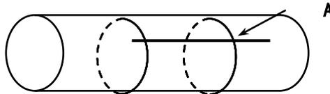
Starting from point A, measure 1/2 of the circumference of the pipe along the edge of the positioning paper. This point is C. Draw a straight line perpendicular to the edge of the positioning paper at point C; (Figure 7)
