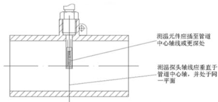
The temperature measuring element is inserted into the central axis of the pipe or deeper
