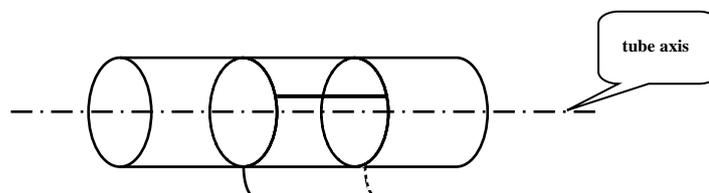
Extend the straight line on the positioning paper to draw a straight line on the pipe; (Figure 5)
