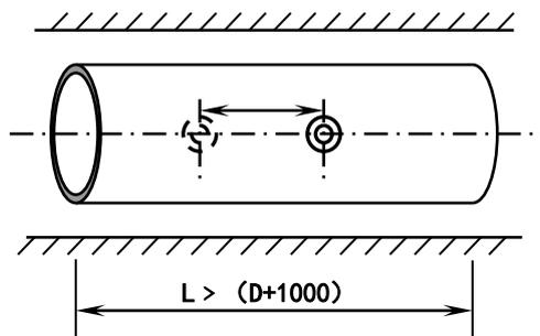
Installing an ultrasonic flowmeter requires a certain straight pipe section, generally greater than 10D upstream, greater than 5D downstream (D is the diameter), and greater than 30D away from
