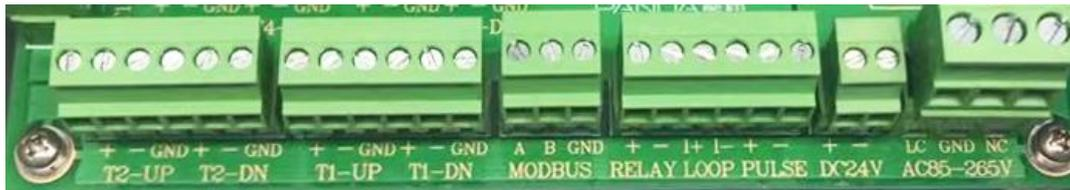
—85-265VAC AC power supply, the power cord is connected to the three sets of terminals corresponding to the picture (GND, LC, NC).
