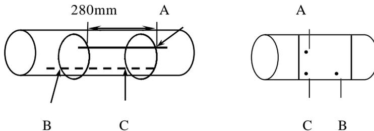
Weld the ball valve base to points A and B respectively.
