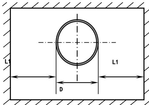
Longitudinal pipe length  $L > (D+1000)$  mm. (Figure 2)
