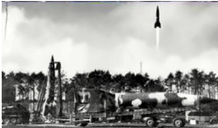
The 14m V-2 rocket is propelled by alcohol & liquid oxygen fuel to an altitude of 90km at a speed of 5400km/h with a range of 320 km & a 740 kg load. All modern rockets including the Saturn V moon rocket are based on the A4 concept.
