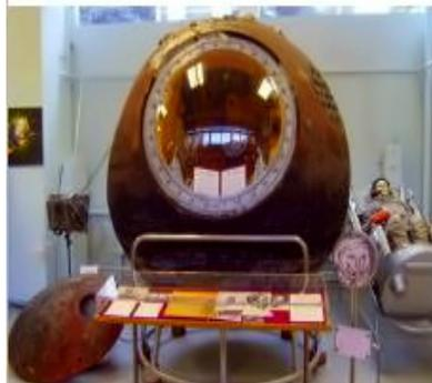
The craft consisted of a spherical descent module (diameter 2.3 meters, mass 2.46 tons), which housed a cosmonaut, instruments, escape system, & a conical instrument module (mass 2.27 tons, 2.25 m long, 2.43 m wide). Holding propellant & an engine system. On reentry, the cosmonaut did eject from the craft at about 7,000 m descend via parachute. The capsule would land separately.
