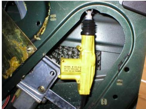
Here is a picture showing the after-market pistol-style actuator ready to be mounted in the rear
