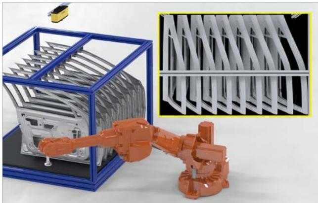
Vision-guided robotics helps move stamped parts from the line to a rack for inspection and identification.
