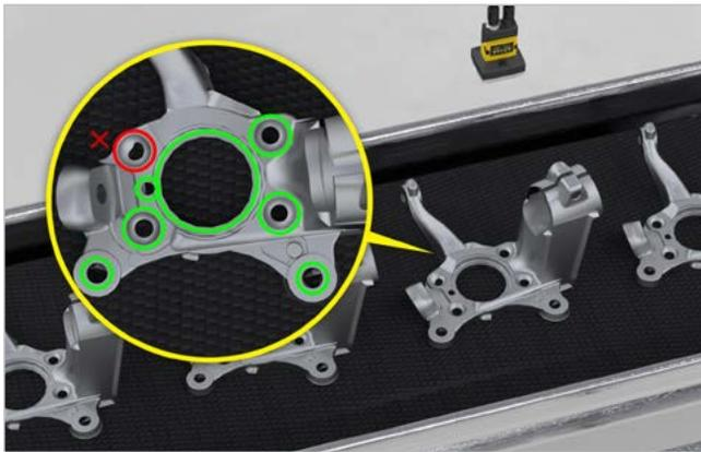
Vision sensors inspect steering wheel knuckles prior to module assembly.
