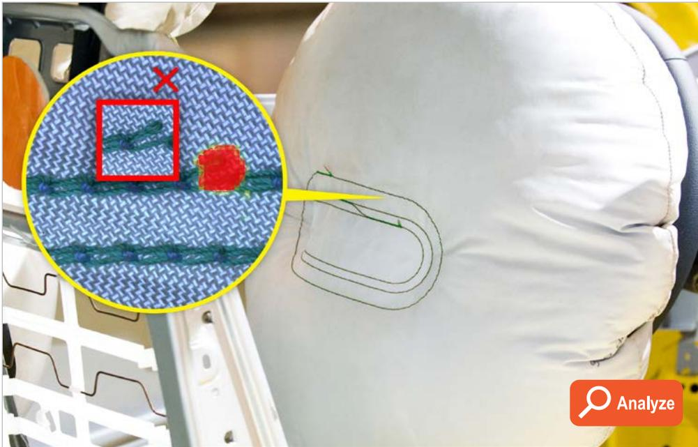
Deep learning vision software inspects the stitching on airbag fabric and stitching for defects.
