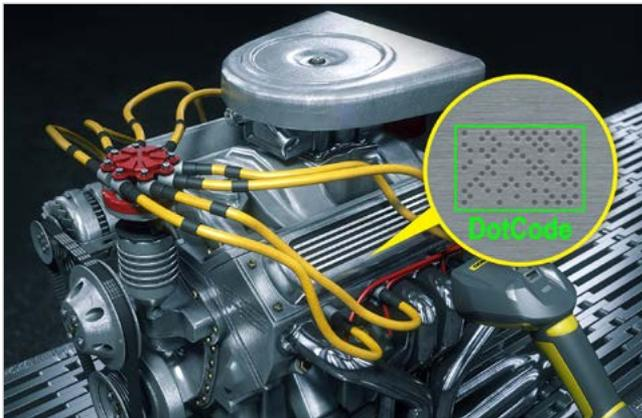
Barcode readers identify components used in the engine assembly.
