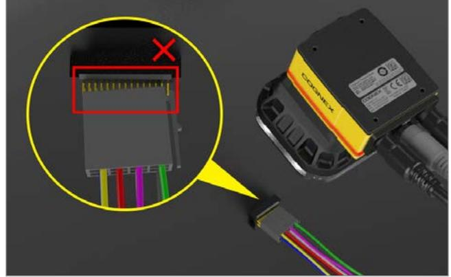
Machine vision systems confirm that wiring harnesses are properly seated.
