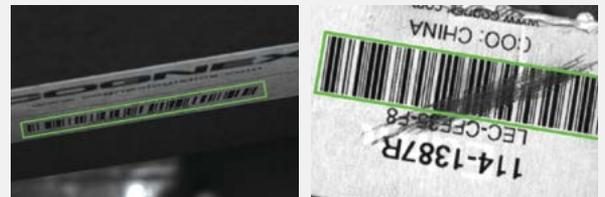
**OCRMax™**, a font-trainable optical character recognition and verification (OCR and OCV) tool, has set industry records for ease of use, read rates and speed in complex images. This powerful algorithm prevents misreads, handles process variations, and provides easy font management.
