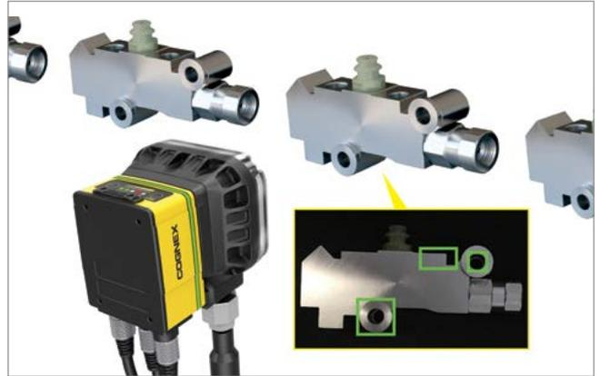
Machine vision systems inspect threads, features, length, and surface finish to verify that valves are made correctly.
