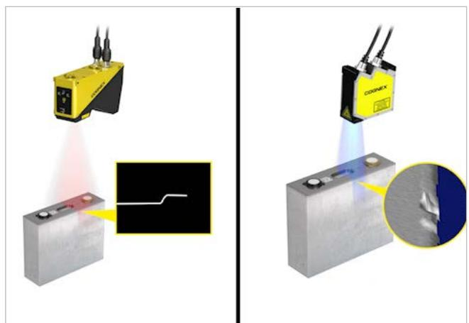
3D laser displacement sensors measure the height difference between the cap and battery case prior to welding. Afterwards, they inspect the welded seams to ensure they are fully sealed and free of defects.
