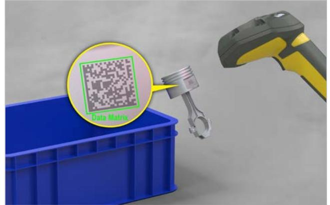
Barcode readers verify that a kit contains the correct parts so vehicles spend less time at each assembly station. This results in more vehicles produced each day.
