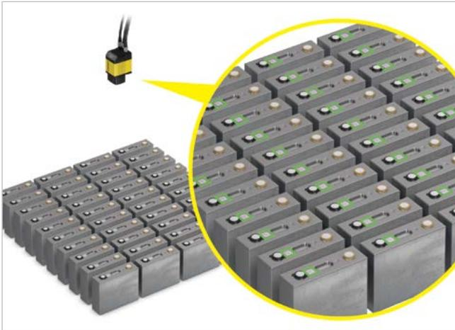
Image-based barcode readers read a large array of codes on battery modules during testing.
