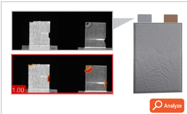
Cognex deep learning vision software identifies defects, such as broken edges, holes, or scratches on the tab's surface.
