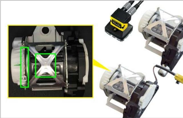
Vision sensors confirm the presence of critical features and dimensions of seatbelt components prior to assembly.
