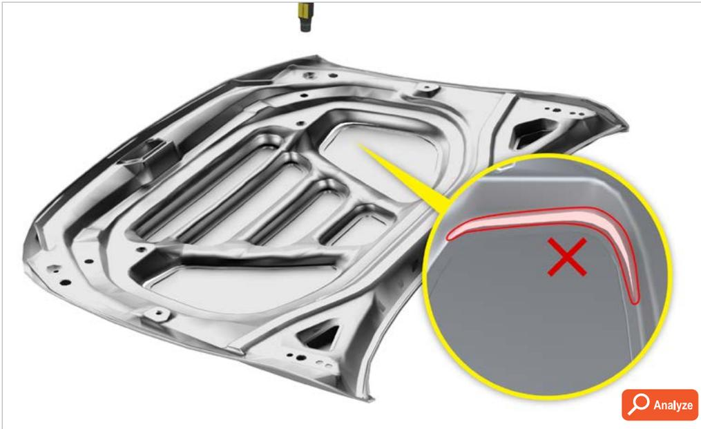
Detect the presence and gauge the width of an opening within a stamped piece of metal.
