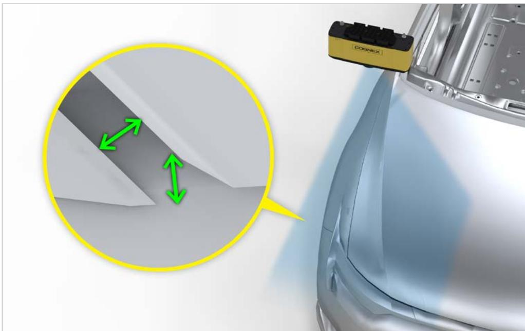
3D vision systems generate an area scan image in x and z dimensions to detect any difference in the height or gap between the two doors.
