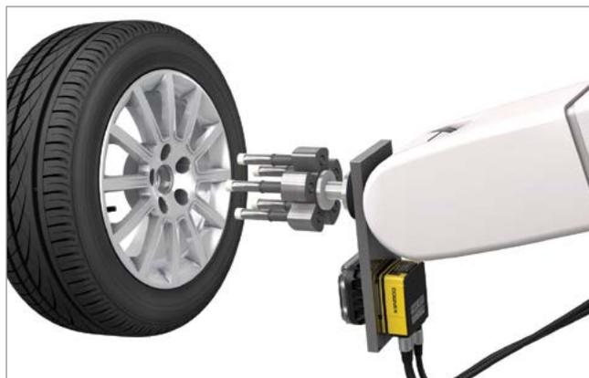
Machine vision systems guide robotic arms to help locate and properly torque a wheel's lug nuts.
