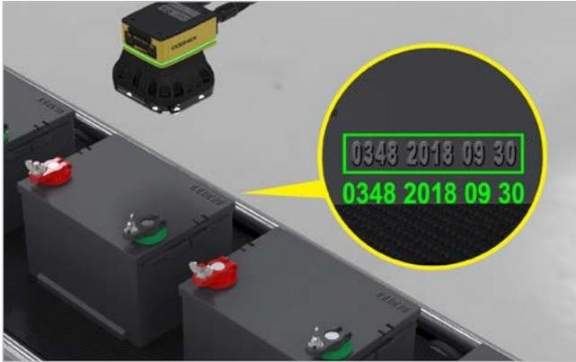
Machine vision systems verify the presence and placement of battery terminals and identify them by their alphanumeric codes.
