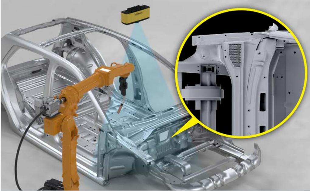
3D vision systems guide welding robots to correct location in order to weld the chassis together.
