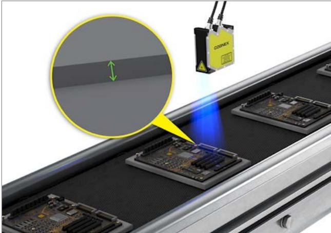
Laser displacement sensors measure the height difference between the carrier and the printed circuit board (PCB) to inspect for warpage. The sensor does this while in continuous motion, speeding inspection.
