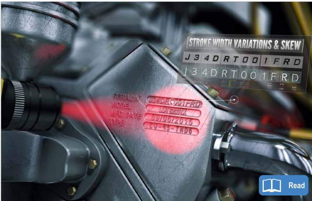
Vision systems with optical character recognition (OCR) read codes to track and trace engine blocks.
