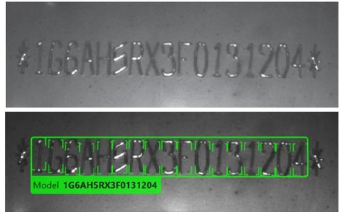
Deep learning vision software reads the deformed characters marked on a VIN code for traceability.
