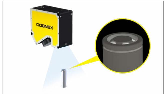
3D laser displacement sensors inspect the dimensions of battery caps to ensure they are fully sealed and free of defects. They use a highly accurate telecentric lens to accurately capture grooves and any defects like tilting or uneven height, regardless of the can's color.
