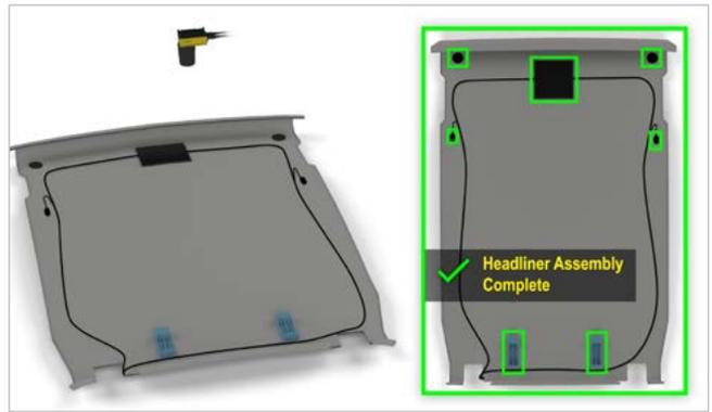
Machine vision systems detect the presence and absence of headliner components and verify the part has been assembled correctly.
