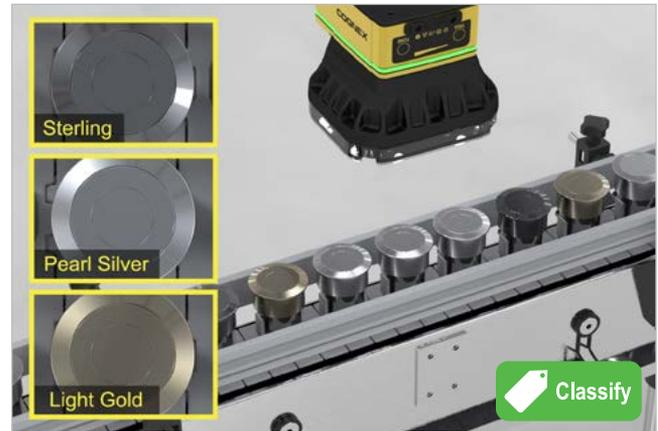
Deep learning vision technology inspects the presence of the proper FPA by color as well as the FPA seal presence and proper insertion.
