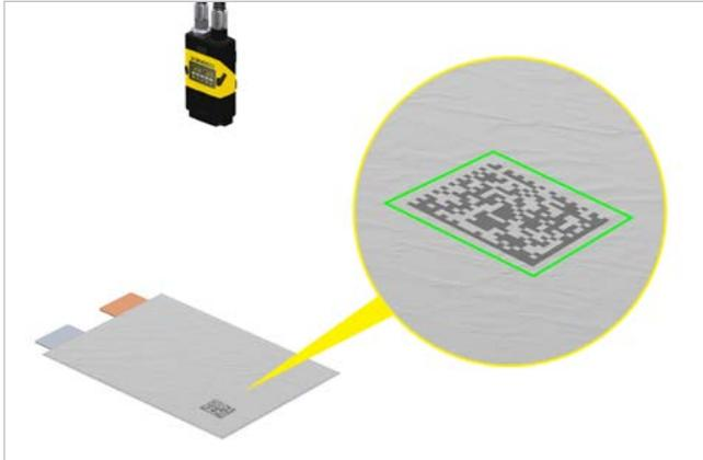
Image-based barcode readers read stretched DataMatrix codes on a pouch's surface.
