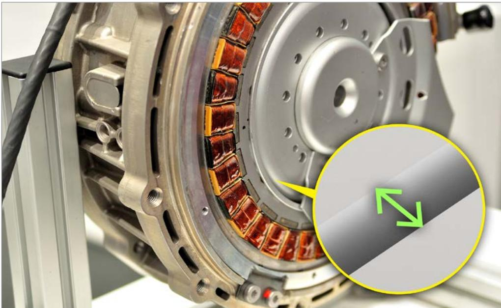
3D laser displacement sensors perform in-line inspection of the narrow gap between rotor and stator, and assesses wedge tightness for the magnetic field.
