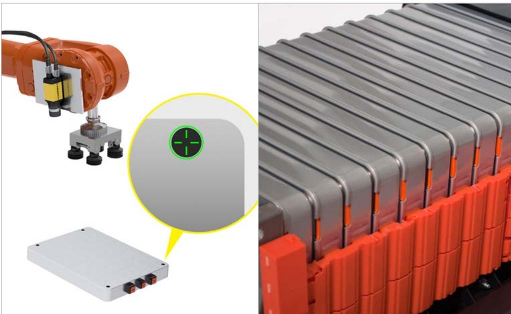
Machine vision systems guide the final assembly of modules and cable connectors into a pack.
