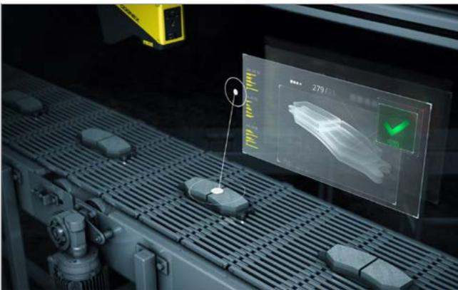
3D displacement sensors inspect brake pad rivets and verify dimensions.
