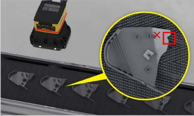
Machine vision systems detect the presence of a short shot, the production of an incomplete part, within 0.5mm.
