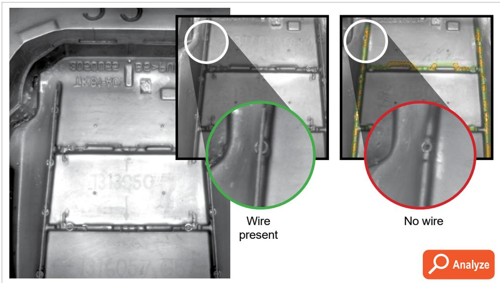
Deep learning vision software verifies the presence of components on a confusing surface during final assembly.
