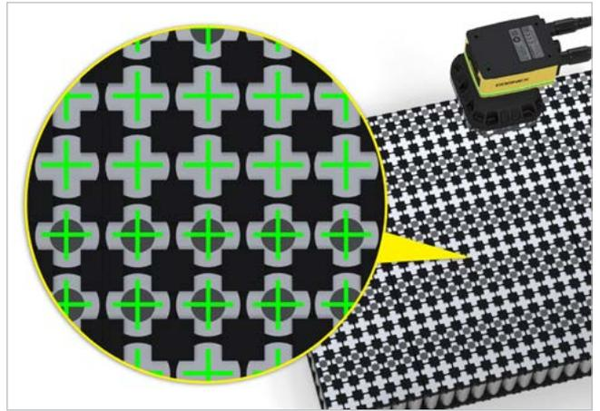
Machine vision systems use geometric pattern-matching to verify battery pack modules are aligned.
