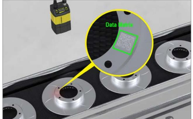
Barcode readers identify components for the brake assembly, even on highly reflective surfaces.
