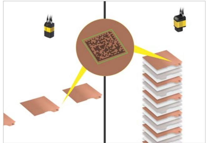
Image-based barcode readers read laser-etched Data Matrix codes on the copper sides of cell sheets and the top of stacked electrodes.
