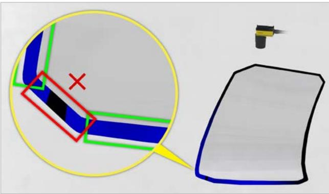
Detect the presence of primer via a UV tracer mixed into the primer; a Pixel Tool along with a measurement tool detects the presence along with the width of the primer area.
