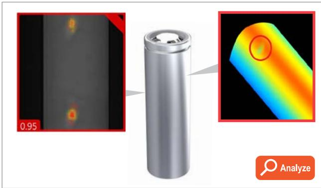
Cognex deep learning vision software detects unpredictable cosmetic defects like dents, scratches, or stains on a cylindrical battery can. Users can stack 2D and 3D images of cells to analyze them simultaneously.
