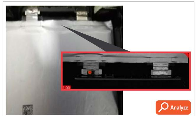
Cognex ViDi deep learning vision software checks welding quality and finds defects like over-welding, missing welds, or burns on tabs.
