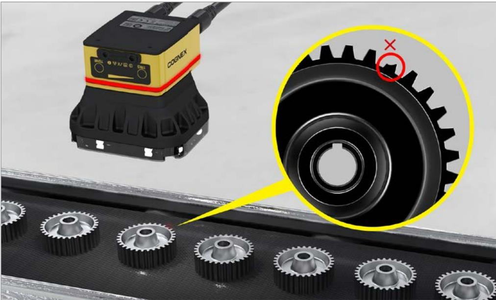
Machine vision systems gauge the dimensions of transmission gears and inspect for damage.
