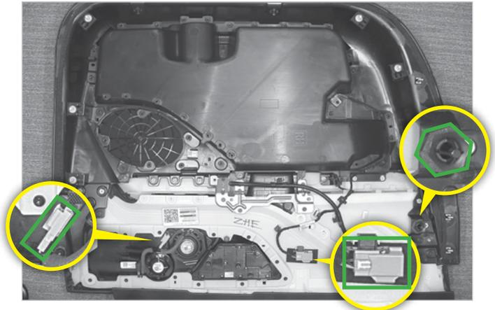
Detect the various door component types, "birds-beak" clip presence, and proper seating, as well as reading most of the barcode labels (flat surface).
