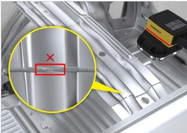
After welding is complete, the number of welds, their location, and absence/presence is verified with visual 2D inspection.
