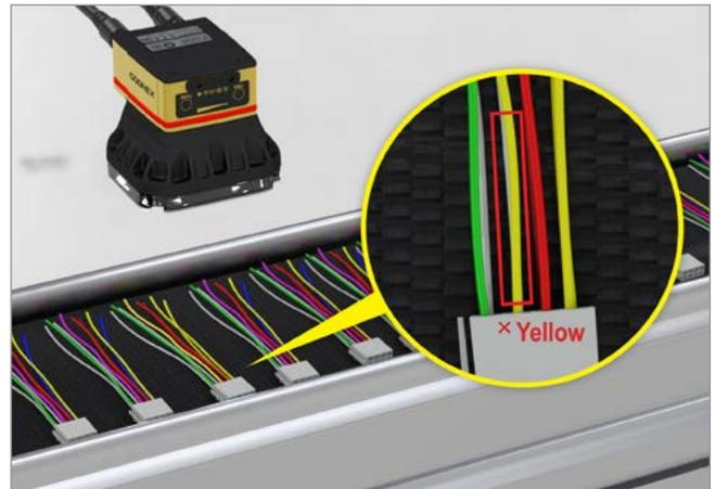
Machine vision systems inspect electrical modules for color and quality prior to assembly.
