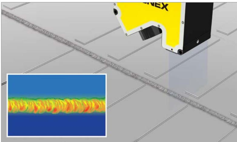
3D laser displacement sensors perform surface measurement of the welds on battery packs. Cognex deep learning vision software helps detect unpredictable weld defects, despite specular glare on challenging metal surfaces.
