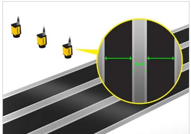
Cognex industrial area scan cameras and VisionPro software gauge the dimensions of the separator and electrode.
