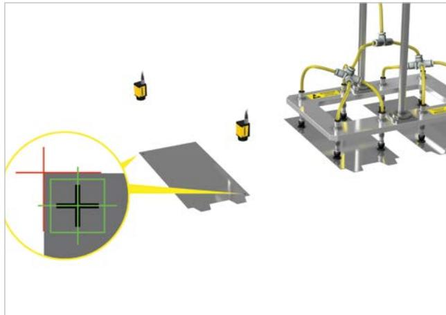
Cognex industrial cameras and VisionPro software align cell sheets for stacking.
