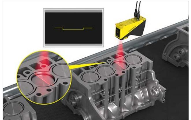
Laser profilers gauge whether pistons are seated properly in a cylinder block.
