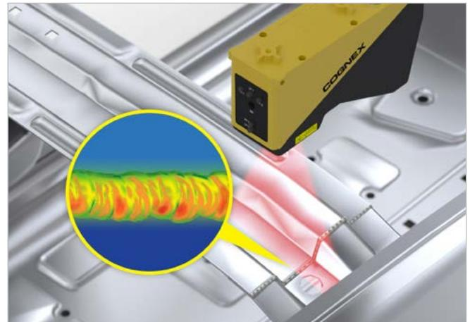
Weld seams are inspected with 3D vision systems to ensure they are complete and the proper thickness.
