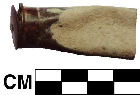
Figure 7: Mechanical damage from iron cup internal primer. Artifact number 48CR480-1503.
