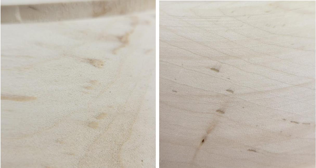
Gouge sharpened with a 600 grit wheel on the left & Gouge sharpened with an 80 grit wheel on the right. Or is it vice versa?
