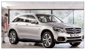
Mercedes-Benz is also showing preproduction models of its GLC F-CELL fuel cell plug-in hybrid. In addition to hydrogen, the all- electric variant of the popular SUV will also run on electricity. With 4.4 kg of hydrogen on board, the preproduction model produces enough energy for a range of up to 437 km (273 miles) in the NEDC, plus up to 49 km (27 miles) of all-electric range using its 13.8 kWh lithium-ion battery. Total output is 147 kW (197 hp) and top speed is electrically governed at 99 mph.
