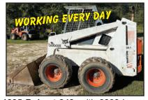
1995 Bobcat 943, with 8000 hours, rebuilt Perkins 4-cyl. (by Perkins dealer), drive pumps and hoses replaced with upgraded units, cylinders rebuilt approx. 100 hours ago, tires replaced with 14-ply heavy-duty sidewalls.....\$15,000 OBO Call 850-527-3547
