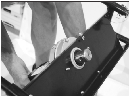
Step 4 - Install motor gearbox on back of mixer frame with flat washers, lock washers and nuts to all 4 studs.
