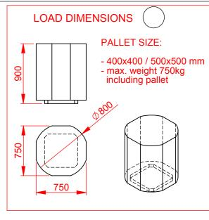
Pallet top surface in loading station approx. 700 - 900 mm
