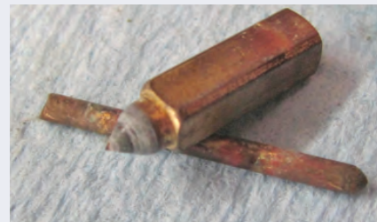
Storing gasoline in the carburetor bowl will result in residue accumulating in the bowl, as shown in the top picture. The Vitron tip float needle was stuck due to tainted fuel, which caused the plastic tip to adhere to the seat of the float needle valve and resulted in a leaking carburetor at start up.
