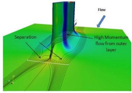
Streamlines around a scAUR<sup>™</sup> fairing around a pier (5) with VorGAUR<sup>™</sup> vortex generators (3) that produce no scouring vortices.
