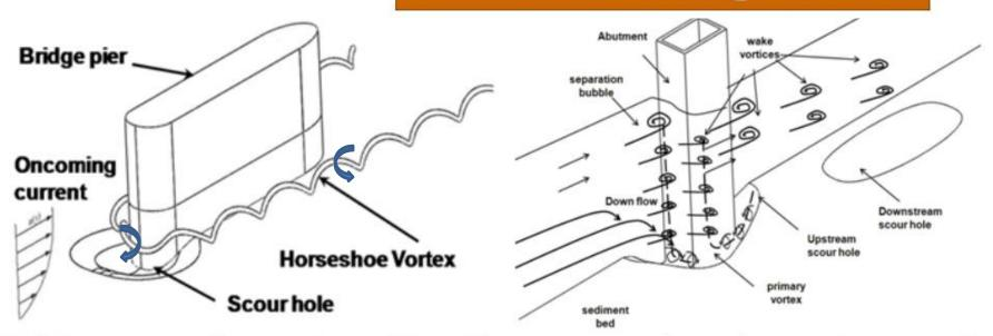
**Bridge scour is produced by discrete vortices** formed around unprotected piers (left above) and abutments (right). Many near catastrophes and loss of life have occurred, as shown in examples **LIKE TORNADOS - VORTEX STRETCHING INCREASES VELOCITY**  $V_2 = V_1(A_1/A_2)^{1/2} = \Gamma/(\pi d_2) = Strength of Vortex/(Perimeter of Vortex)$
