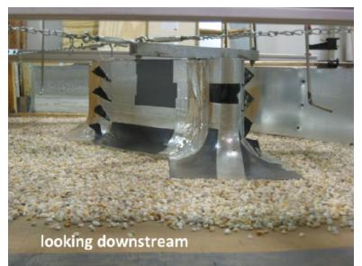
(left) Upstream view showing location of VGs on model front right and rear left sides. (right) Laser sheet showing no scour downstream of the model.
