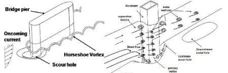
Bridge scour is produced by discrete vortices formed around unprotected piers (left) and abutments (right)
