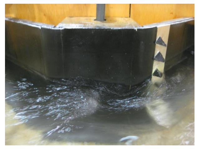
View of case #20 modified wing-wall abutment model with VGs. Note the free surface height change after the contraction due to the surface vortex.
