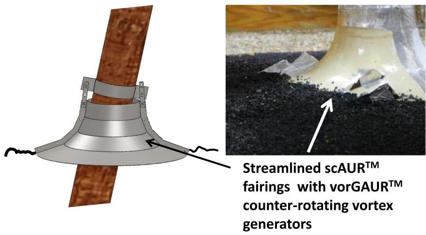
Proven principle of scour research – if it does not scour at model scale, it does not scour at full scale for the same sediment size
