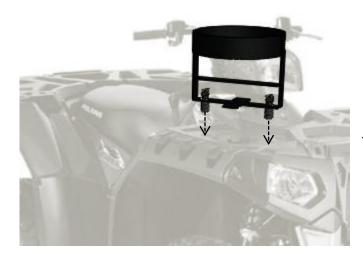
Insert the 5 Gallon Bucket Holder into the chosen location by aligning the anchors with the holes on the Front or Rear of the Sportsman.
