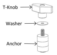
Remove the T-Knob and Washer from each of the Anchor Assemblies.
