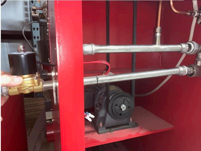
6. Remove plastic gaskets so as not to lose them. The turn gas valve sideways to put it out od back of roaster:
