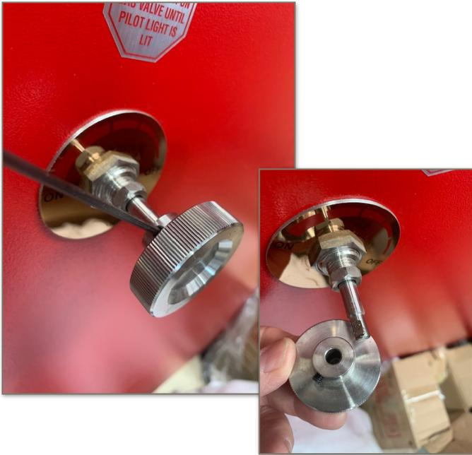
1. Using a Metric Hex ket remove the metal handle
