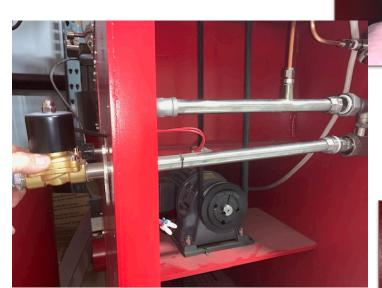
6. Remove plastic gaskets so as not to loose them. The turn gas valve sideways to put it out od back of roaster:
