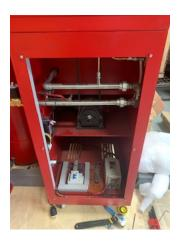
In the rare even your Needle gas valve becomes hard to turn use Penetrating Lubricant and spray into front of shat & allow to sit for at least 10 minutes. Then turn some. Repeat until you can turn valve completely.
