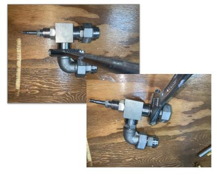
8. Now replace with new valve and follow exact procedure in reverse. On these two gas lines that hook directly to the valve use yellow gas tape or white teflon tape if you don't have gas tape or joint compound or Leak Lock on the threads of fittings before attaching to gas valve.
