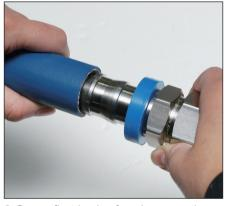
2.Cover first barb of end connention with hose.( Lubrication fitting stem with light oil may ease assembly)
