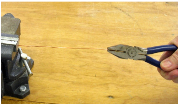
Pulling to straighten a bent wire
