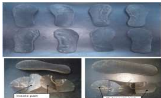
Fig. 3. Prepared tyre outsole
