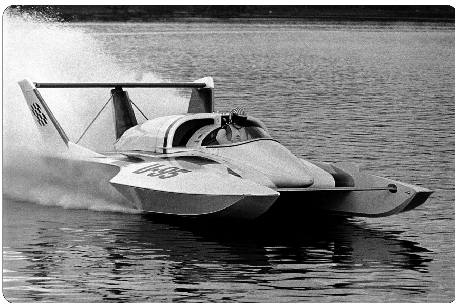
Billy Schumacher was involved in the early stages of the U-95 project, which resulted in the first successful use of a turbine engine in an Unlimited.
