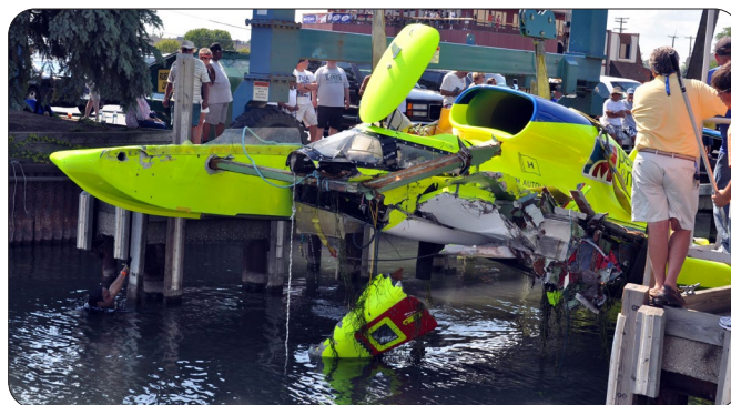
The U-37 Miss Peters & May hits the wall at Detroit in 2010. TOP: The boat's skid fin has broken off. MIDDLE: A fraction of a second before hitting the wall. ABOVE: The damage. The left sponson and part of the cockpit were demolished. Driver J.W. Myers suffered a broken foot.
