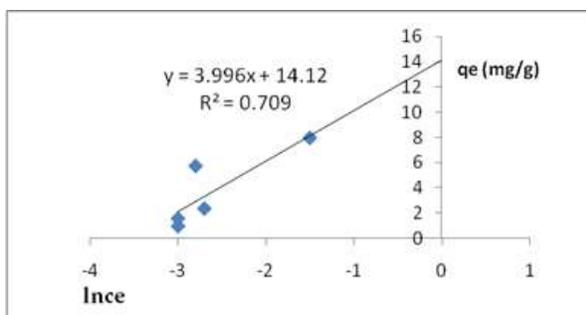
**Figure 8.** Temkin isotherm model for cadmium (II) adsorption.
