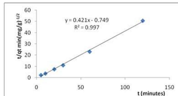
**Figure 11.** Second order kinetics for cadmium (II) adsorption.
