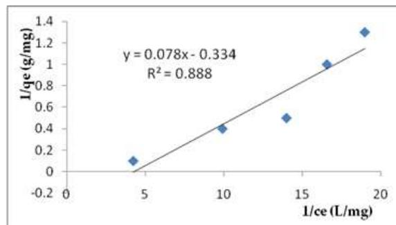
**Figure 6.** Langmuir isotherm model for cadmium adsorption.
