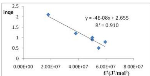
**Figure 9.** D-R isotherm model for cadmium (II) adsorption.
