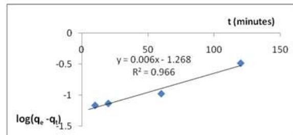
**Figure 10.** First order kinetics for cadmium (II) adsorption
